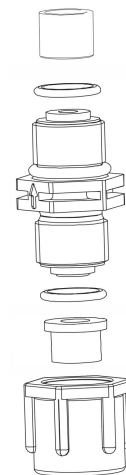
Figure 1: Assembly drawing of the outlet valves (above pump head) and the inlet valves (below pump head).
